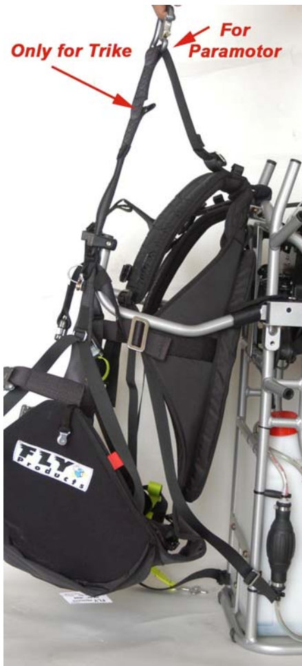
Fig. 15 - Lower harness attachment
